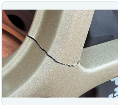
Physical crack / root transition
